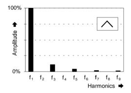
Fig. 4: Harmonic spectrum of a triangle wave
