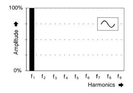
Fig. 5: Spectrum of a sine wave
