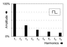
Fig. 3: Harmonic spectrum of a true square wave
