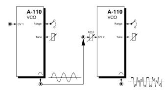
When you try this out (see Fig. 8), start off with sine waves, and slowly raise the modulation frequency from the sub-audio into the audio range.
