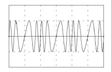
**Fig. 6:** Frequency modulation using a slow LFO (Vibrato)
