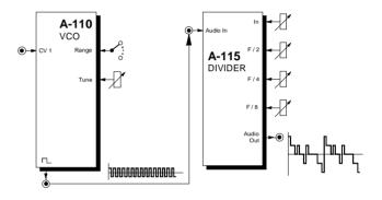
Fig. 12: Using the DIVIDER to add sub-octaves
