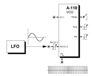
Fig. 11: Pulse Width Modulation using an LFO
