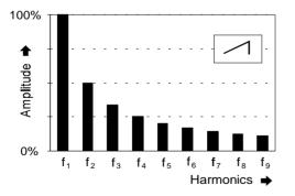
Fig. 1: Harmonic spectrum of a sawtooth
