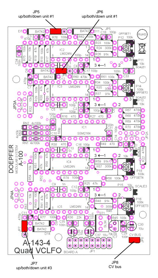
JP5 ... JP7: The jumper positions shown correspond to "up". If the jumper is installed at the other position the function is "down". If the jumper is removed the function is "both".
