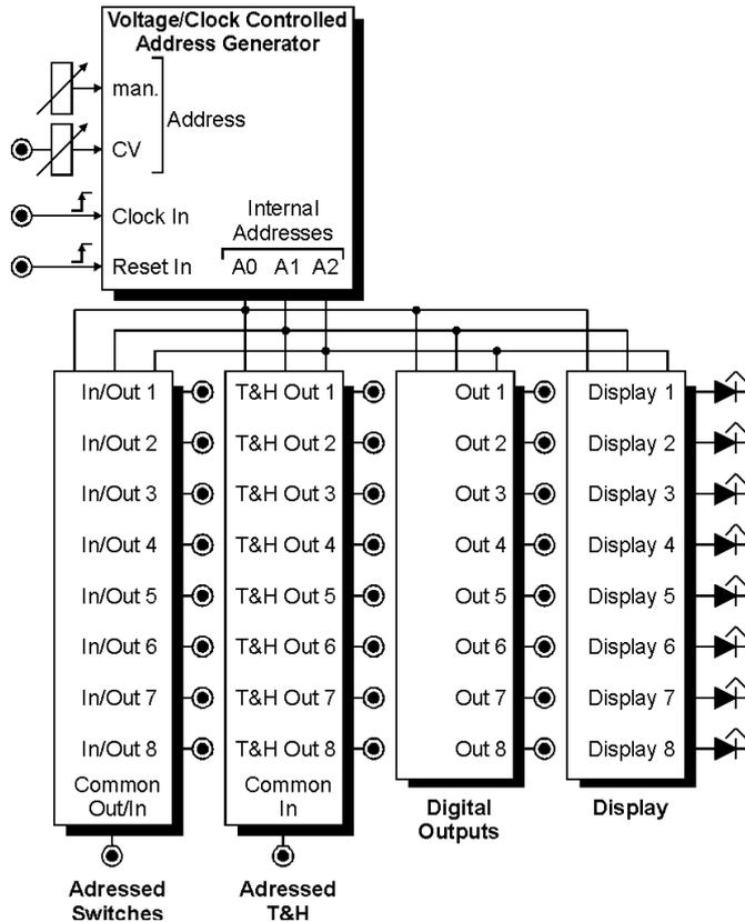
Module A152 is a useful switching and Track&Hold module. It combines three sub-units within one module:
