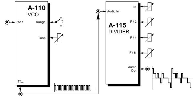
Fig. 12: Using the DIVIDER to add sub-octaves
