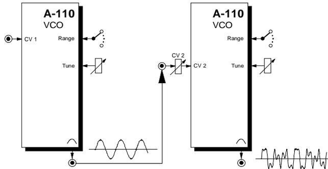
**Fig. 8:** Frequency modulation in the audio range
