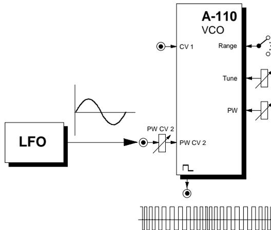
Fig. 11: Pulse Width Modulation using an LFO
