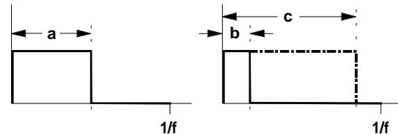
Fig 2: Square waves with different pulse widths
