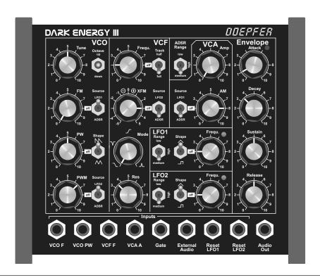
As soon as the power adaptor has been plugged in, Dark Energy III will power up. The LEDs in both LFO sections will now light up and alternate between red and green. The LED on the back panel will flash intermittently for about two seconds and then stay lit permanently.
