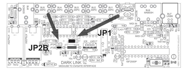
To generate a switch trigger, the jumper (JP1) has to be taken off.
