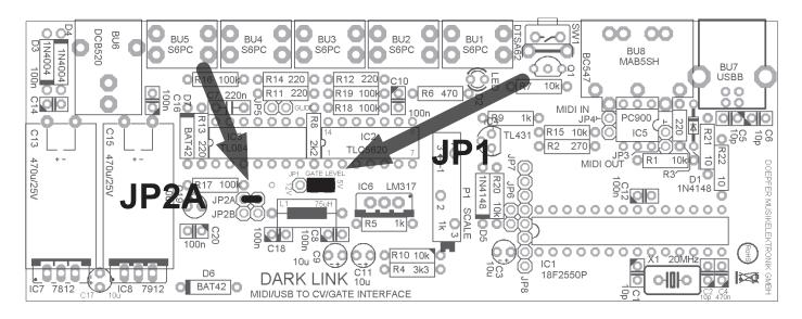
JP1 position for 12 Volts trigger (middle and leftmost contacts)
