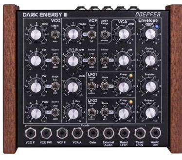
Dark Energy III is the successor of Dark Energy II. The main differences between II and III are an improved VCO (no warm-up period, additional triangle waveform, wider frequency range), resettable LFOs, improved ADSR and a lot of internal access points for DIYers. The favored filter of the Dark Energy II has been unchanged.
