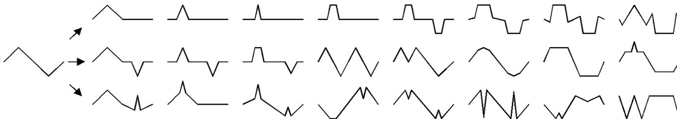
**Fig. 2:** Examples for new waveforms derived from a triangle input with different parameter settings
