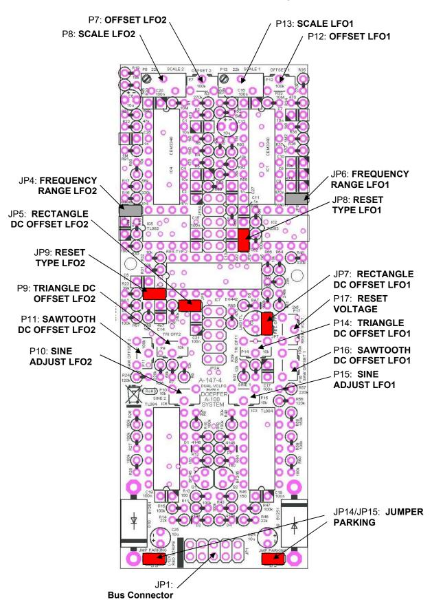
The grey marked jumpers JP4 and JP6 are not installed in the factory. If required the dummy jumpers of JP14/JP15 can be used.
