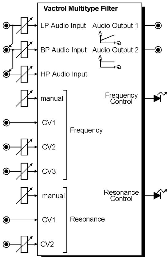
Module A-101-1 is a special **multitype filter** based on an idea by Nyle A. Steiner from the year 1974. Injecting an audio signal into different points of a standard low pass filter circuit leads to the three filter types **low pass (LP)**, **band pass (BP)** and **high pass (HP)**. For **each filter type** a **separate input** is available and the sum of the three filtered signals appears at the **common output**. Even a **notch filter** can be realized.
