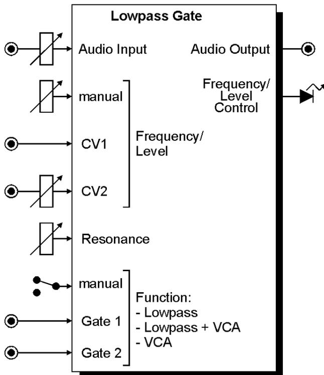
Module A-101-2 is a **vactrol based combination of Low Pass filter (LP) and VCA**. Additionally a combined mode LP+VCA is available. In this mode the sound becomes more dull as the loudness decreases. The A-101-2 was inspired by module 292 of Don Buchla. He also introduced the term "**Low Pass Gate**" for this combination of functions.
