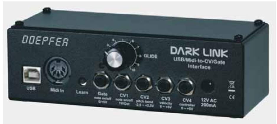
Dark Link is a Midi/USB-to-CV/Gate interface to control vintage monophonic synthesizers via Midi or USB. **Dark Link** is nothing but the USB/Midi interface of the Dark Energy. It has available 4 analog control voltage outputs (CV1...4) and one Gate output.
