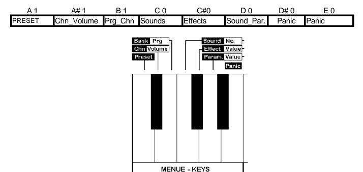
To adjust the parameters the remaining keys of the keyboard are used. The remaining keys are divided into two main groups: **preselect keys** and **value/number keys**
