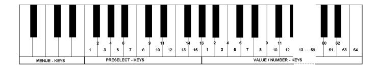
There are **7 menus** available which are selected by means of the 8 MENU-keys in combination with the two buttons part 1 and 2.
