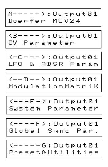
Turning the MENU control moves between the pages. Turn the MENU knob anticlockwise until the screen below is shown. (If you are into a deeper menu, you will need to press the MENU knob to return to this page.
